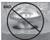
OVAL NECK OF BOLT NOT SEATED PROPERLY
