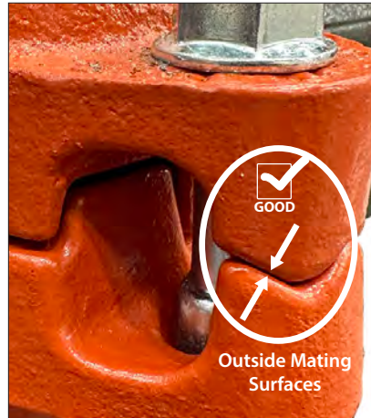
PROPERLY ASSEMBLED JOINT – METAL-TO-METAL CONTACT AS INDICATED AT ALL OUTSIDE MATING SURFACES
