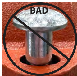
OVAL NECK OF BOLT NOT SEATED PROPERLY
