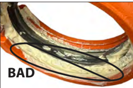
BAD - EXCESSIVE LUBRICANT
