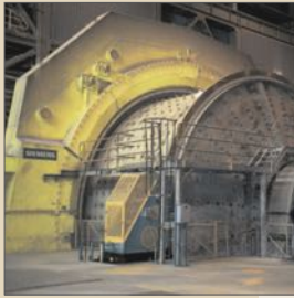
SAG mill at large copper mine in Chile
