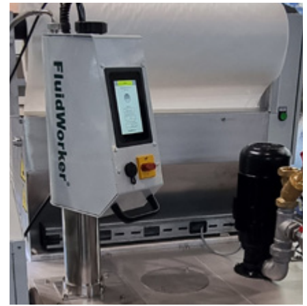
FluidWorker® 50 is installed on the coolant tank.
