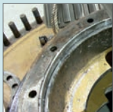
Pitting on bearing
